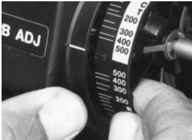
Figure 3-2. Changing Controller Action on 4195KA Series Controllers
