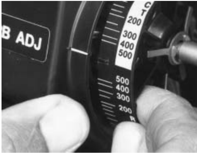
Figure 4-2. Changing Controller Action on 4195KB and KC Series Controllers
